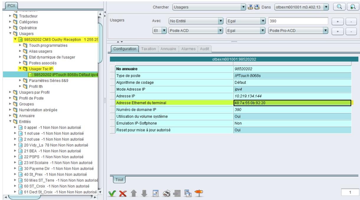
The screenshot shows the PCX software interface. On the left, a tree view shows the navigation structure, with 'Usager Tsc IP' selected. The main window displays the configuration for the user profile '98520202 IPTouch 8068s Défaut ipv4'. The 'Adresse Ethernet du terminal' field is highlighted in yellow.
